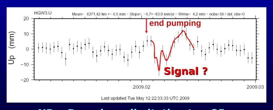
NB Drawdown limitation to <25-30 m because of seawater intrusion hazard may mean weak signal
